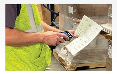
With Barcom's help, Coastal integrated their new Android operating system with their existing ERP system and new, more modern barcoding equipment to streamline the receiving process. With the Honeywell Dolphin CT60 Handheld Computer, workers assign a barcode to each purchase order, and receiving personnel scan that barcode using the mobile computer. A mobile printer will print a label identifying the item and lot number before being affixed to the box or pallet.
